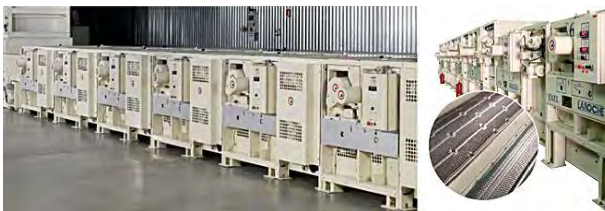
Figure 3: Example of a tearing line from LAROCHÉ designed for recycling of hard textile waste, consisting of 6 opening sections. ( https://www.laroche.fr/en/domaines-dactivites/recycling.html )
