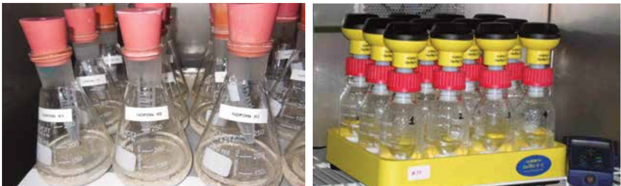
Figure 4.1: Laboratory tests: (a) closed bottles of the sublittoral water-sediment interface lab test, measuring the development of CO 2 ; and (b) incubation bottles of the pelagic (water column) lab test to measure O 2 consumption. (Weber et al., 2015).
