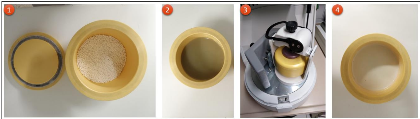
Figure 5. (1) Zirconium dioxide cup with zirconium dioxide balls; (2) filled with montmorillonite pre-dispersion; (3) planetary ball mil; (4) final montmorillonite dispersion after milling
