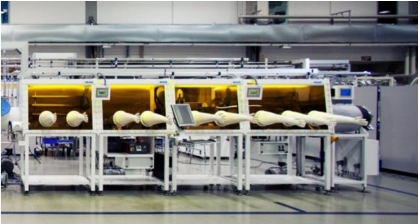
Figure 4: Picture and scheme of sheet-to-sheet ALD unit
