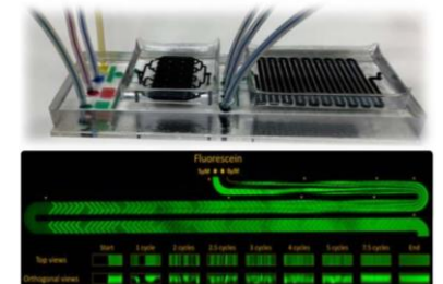
Prototype of a gut-on-a-chip model of intestinal digestion at INL
