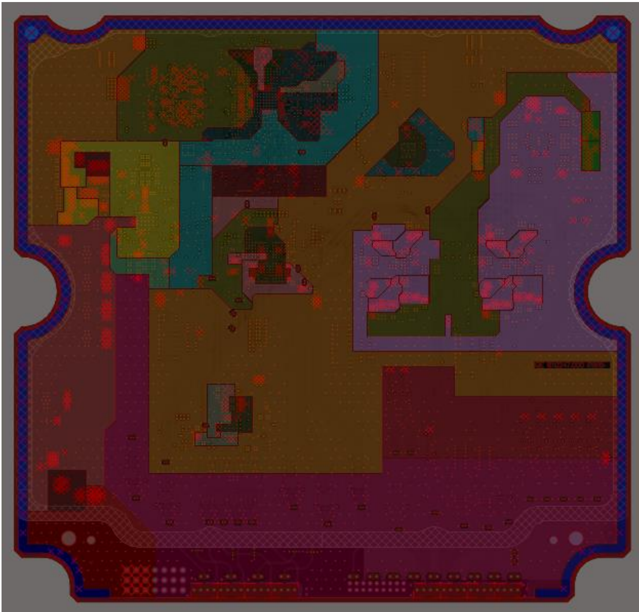
Abbildung 23: D(C) Layout, Powerplane PWR5
