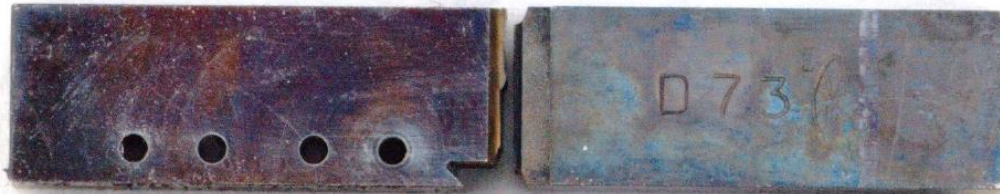
Figure 3: Placement of the starter bore holes for EDM
