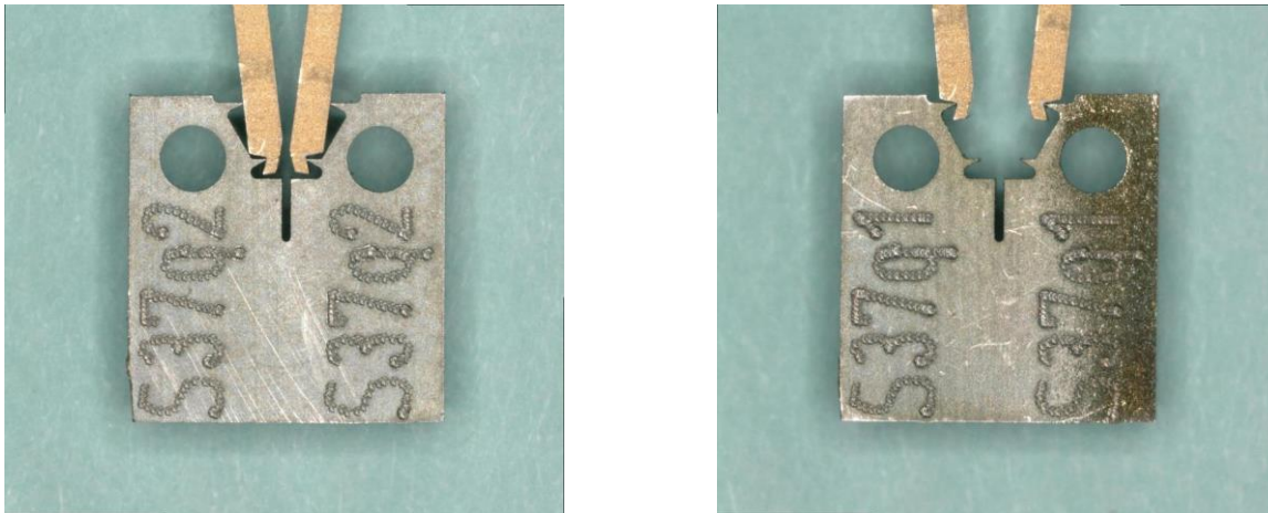
Figure 5: 0.16T C(T) design discussed at Framatome GmbH
