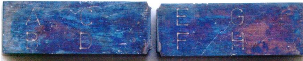
Figure 2: Re-stamping of sample D73
