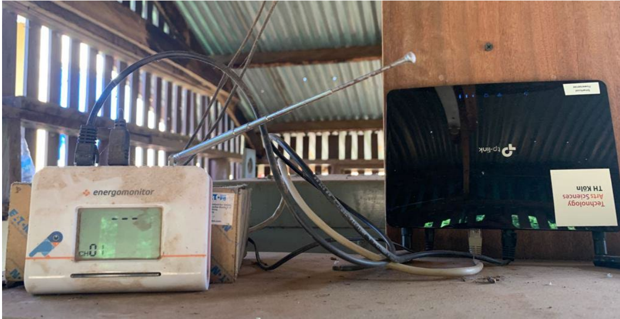
Figure 4 SmartCost Hub connected to mobile router
