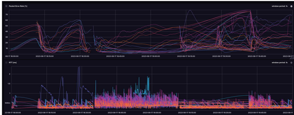
Abbildung 11: MTU Lasttest-Messwerte (Packet Error Rate, Round Trip Time)
