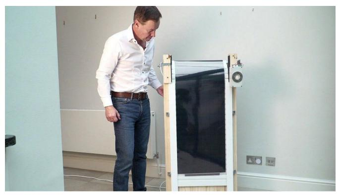
Filia's prototype solar roller blind could be fitted to flats and garages
