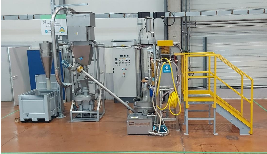
Figure 13: Washing module (left: dryer & cyclone, right: washing tank)
