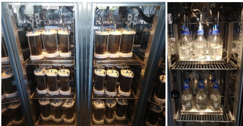
Figure 20: Respirometers for biodegradability assessment, left: in compost condition, right: in marine environment
