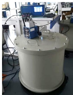
Figure 21: Thermally insulated tank for self-heating disintegration in composting conditions (pilot-scale)
