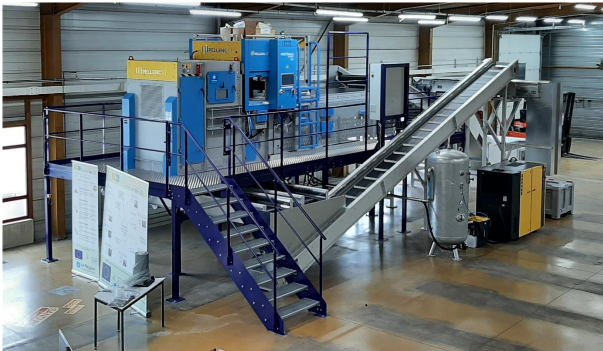
Figure 10: Mistral + Connect Near Infrared Optical sorting (Pellenc ST)
