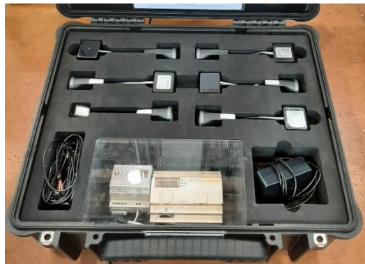
Figure 3: GulPlug equipment for energy consumption measurements
