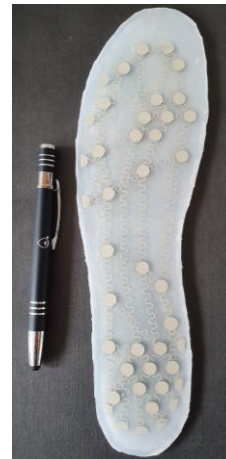
Printed pressure sensors in shoe inlay
