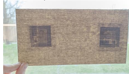
Temperature sensor embedded in flax composite material
