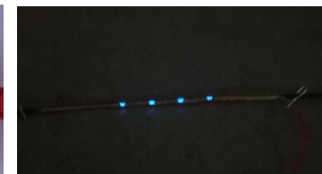
Printed Zinc-Manganese Dioxide battery (1.6 V)
