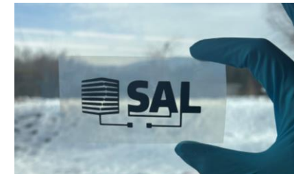
Printed Zinc-Manganese Dioxide battery (1.6 V)
