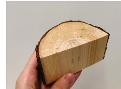
Printed humidity sensor on wood
